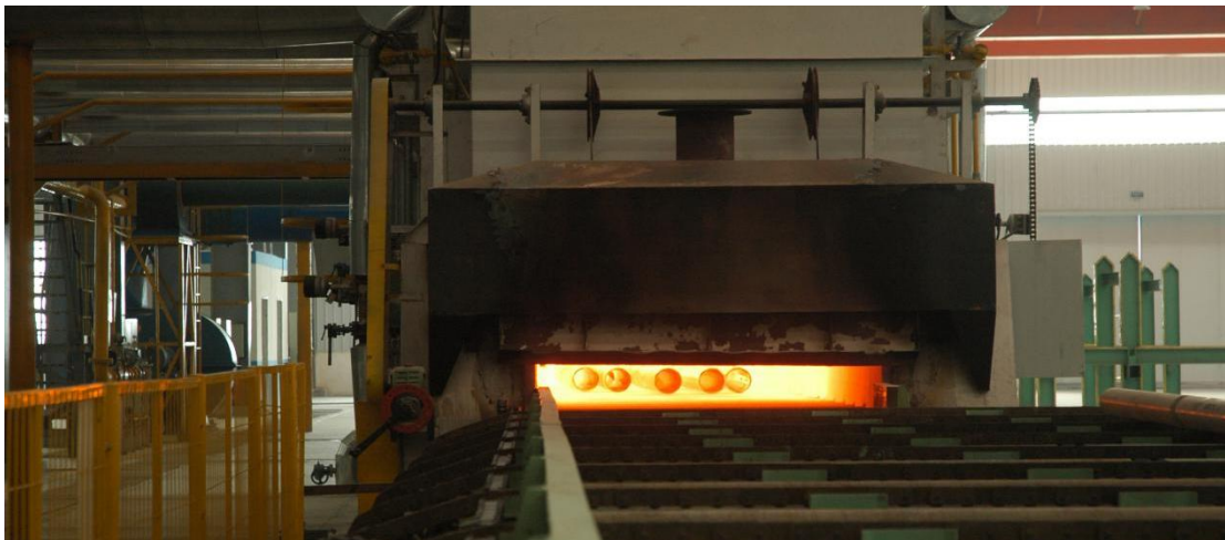
Heat treatment equipment (solution heat treatment)
