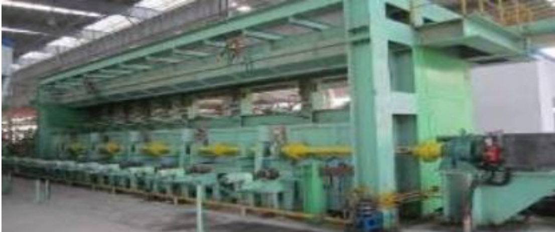
Heat treatment equipment (tempering furnace)
