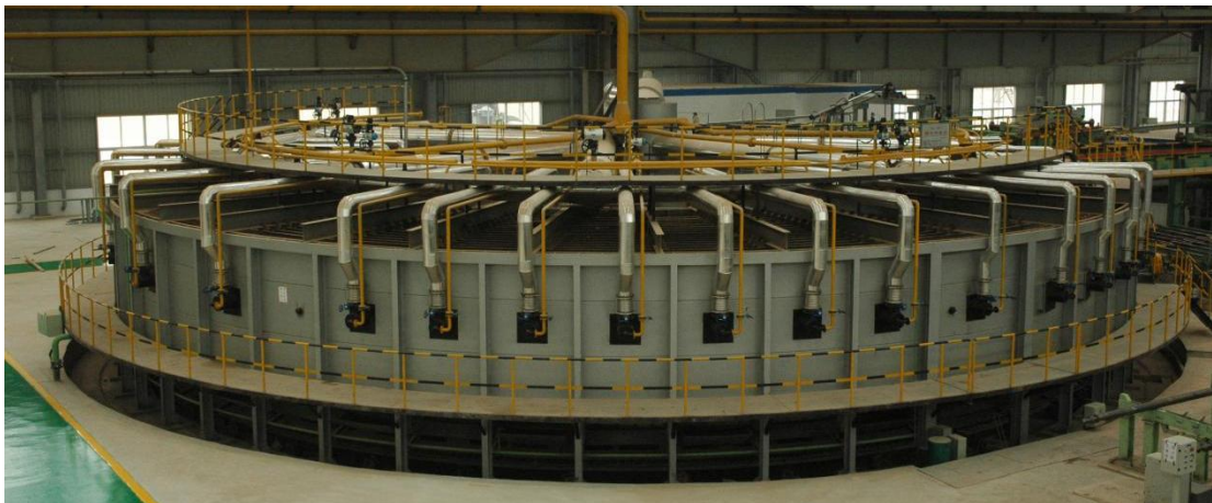
Heating furnace (ring)
