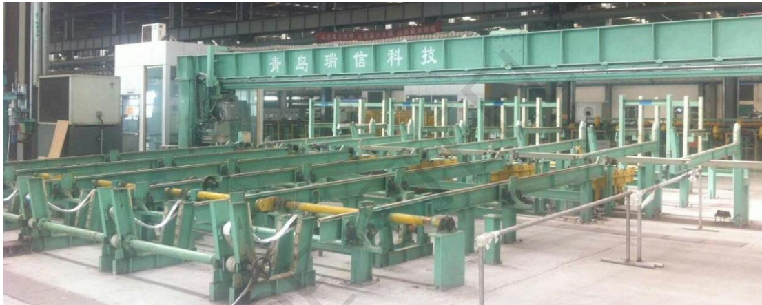
Online automatic marking equipment
